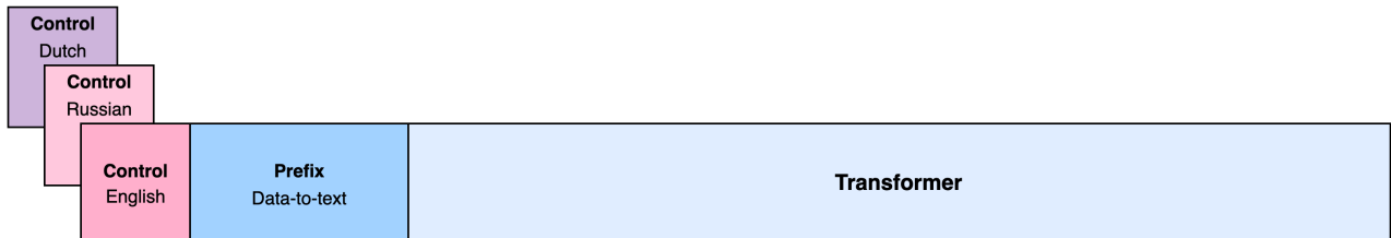
Figure 2.1: Visualisation of four parameter tuning techniques. Firstly there is fine-tuning, where all parameters of a large Transformer LM are updated. Secondly, prefix-tuning updates a task- and language-specific prefix while keeping all LM parameters frozen. Mixed prefix-tuning combines regular prefix-tuning with a discrete prompt, allowing a single prefix to learn a task in multiple languages. Lastly there is the language control prefixes approach, updating both a general task prefix and a language-specific prefix.
